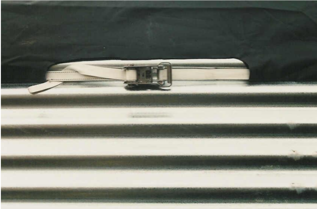
Image 3: pull the ratchet buckles tight
